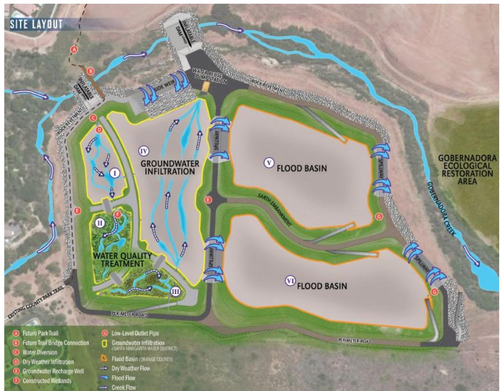
a measure to respond to the existing erosion and sedimentation problems along Gobernadora Creek, as well as to provide detention to the high storm flows damaging downstream restoration habitat areas, arrest the excessive surface and groundwater originating upstream, and improve the degraded water quality along Gobernadora Creek. OCPW became a project partner to maintain operations of the lower basin for flood control functions.
