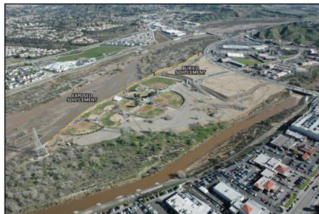
Figure 13. Aerial view of Hart Baseball Fields, Santa Clarita, CA during January 2005 storms
